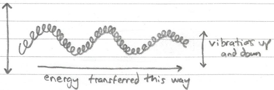
Examples of transverse waves include Light and the electromagnetic spectrum, water waves and some earthquake waves.
