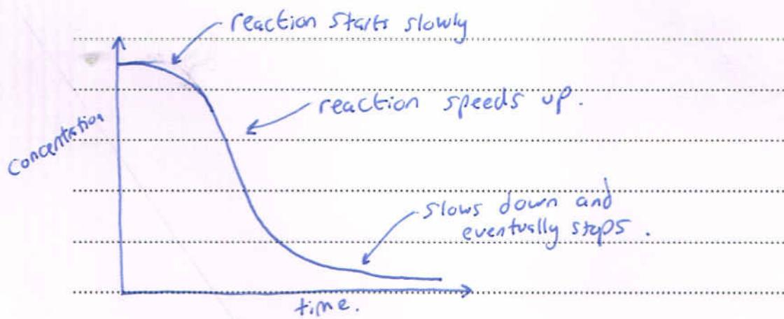
At start curve has a small gradient showing a slow rate. This is because at the start negative ions are colliding, which gives a very high Eq. However as reaction progresses  $Mn^{2+}$  ion form which autocatalyses the reaction speeding it up. Eventually reaction stops as  $MnO_4^-$  ions are used up. (5 marks)
